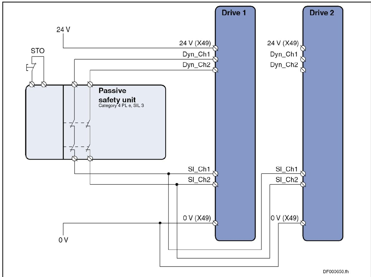
Fig.7-7: Example zone formation (here: 2 IndraDrive Cs in a safety zone with two-channel wiring and passive safety unit)
