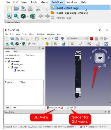
To create one of the six views, orient the model in the desired view, and press "ctrl-A" to select all. In the TechDraw menu, select "Insert View". This will create a "View" under the "Page" created earlier.
