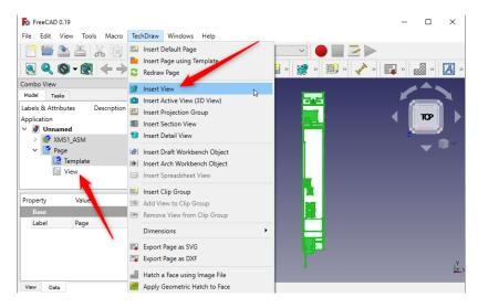
Change the orientation to another of the six views, press "ctrl-A" to select all and select "Insert View" from the TechDraw menu. Repeat this process until all six views are created. Each new view is put in the center of the page, overlapping the first view. After each view is "inserted" return to the page view and move the new view to the side where it will be visible. The end product should up looking like this:
