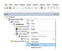
2. Select the Ethernet-Device provided by the node *Fieldbuses -> Ethernet Adapter* and press button *Add Device*.
