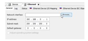
The available network adapters on ctrIX CORE are shown afterwards. Select the network adapter for the fieldbus communication and confirm by pressing button *OK*.
